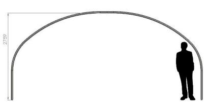
The hoops, ridge bar and corner braces in this model are 50.8mm diameter high tensile steel tube. 1.35m long foundation tubes sleeve inside the straight leg by up to 600mm for structural support.
